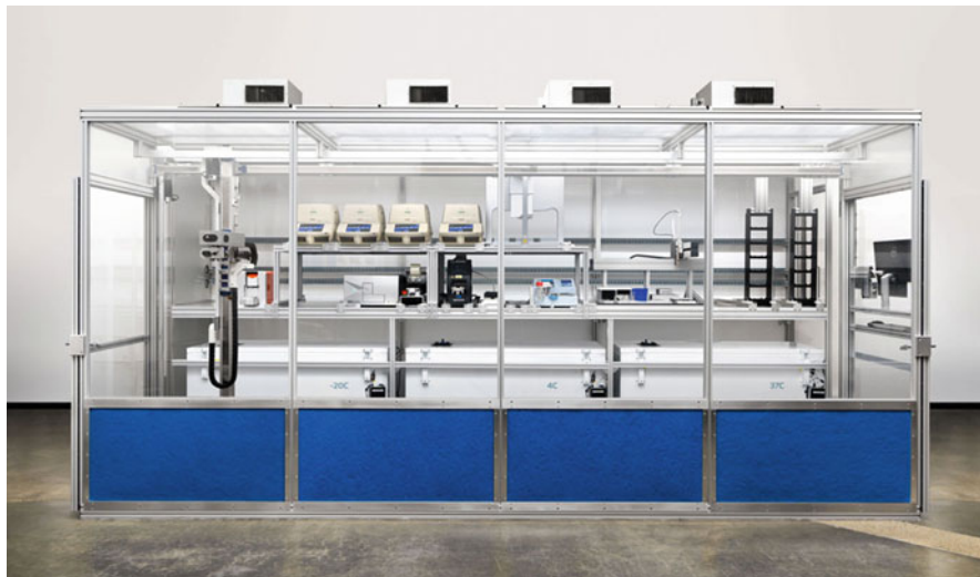
Fig. 11.12 Transcriptic Workcell, a custom robotic cellular and molecular biology laboratory. (Image adapted from https://www.transcriptic.com/ )
